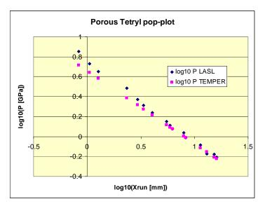
Figure 10: Pop-plot of porous Tetryl (density = 1 500 kg/m3) Experimental pop-plot (dark blue) and values from a fitted Yactor's model (pink)
