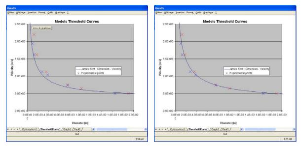
Figure 9: Flat steel projectile on bare PBX9404 two sets of parameters: James (Right) and TEMPER (Left)
